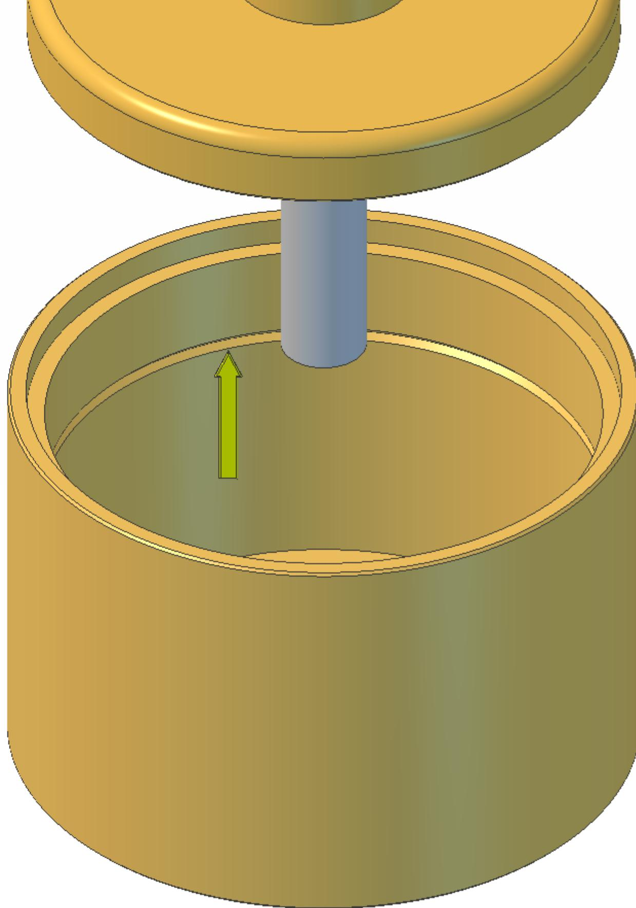
Fit the burner cap into the burner body.
