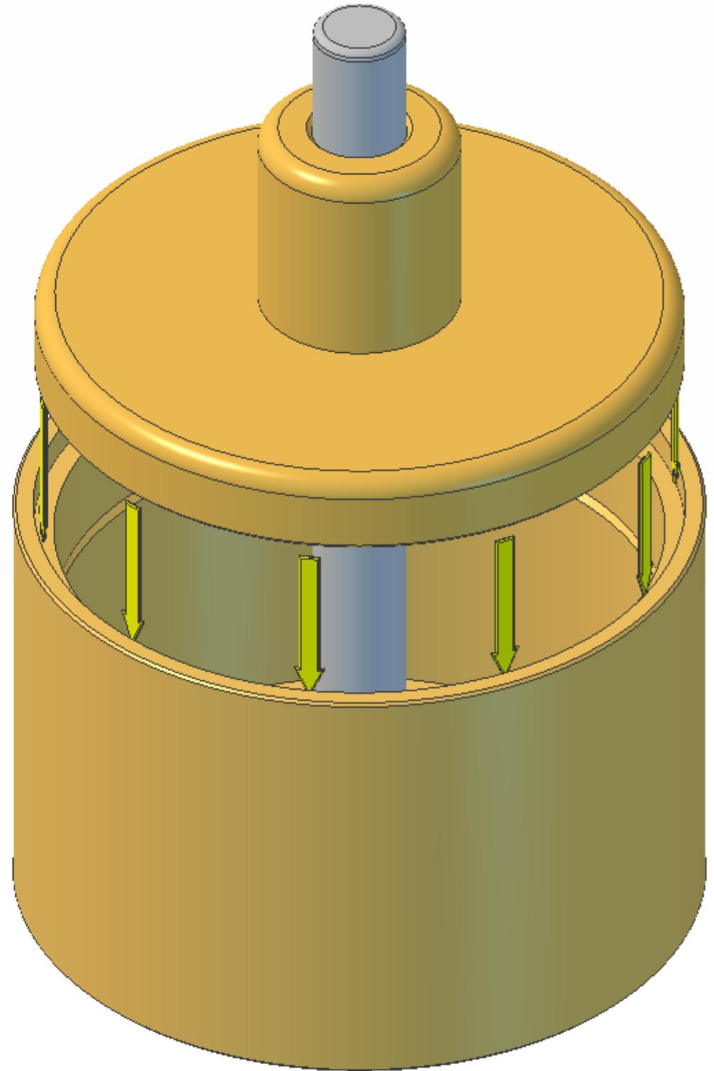
Fit the assembled burner into the hole in the plate.
